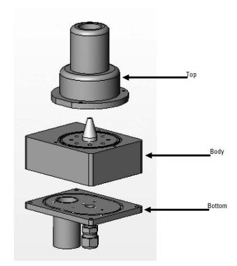
Figure 10-1. Exploded view of the virtual impactor.
