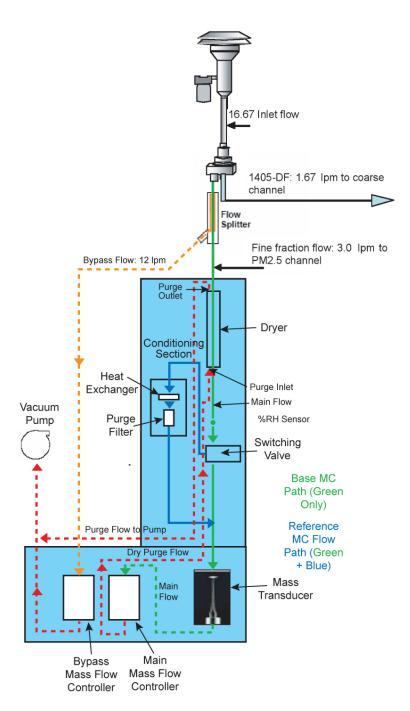
Figure 3-2. Schematic representation of the Base MC and Reference MC flow paths for the  $PM_{2.5}$  sample air stream. A parallel system operates simultaneously for the PM-Coarse sample air stream in the 1405-DF. (Original schematic courtesy of Puget Sound Clean Air Agency.)
