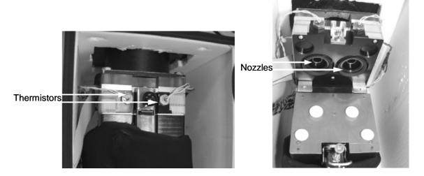
Figure 10-5. Air Inlet containing the Mass transducers, thermistors, and nozzles.
