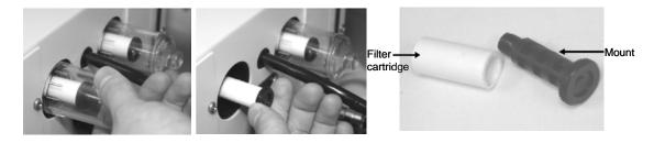
Figure 10-3. The  $PM_{2.5}$  and PM-Coarse in-line filters should be changed every six months.
