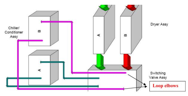
Figure 9-6. Isolate the chiller by "looping the elbows".
