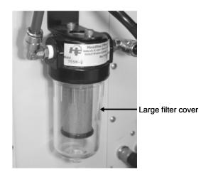
Figure 10-4. The bypass flow in-line filter should be changed every six months. This coalescing filter also serves as the water trap on the 1405-DF.
