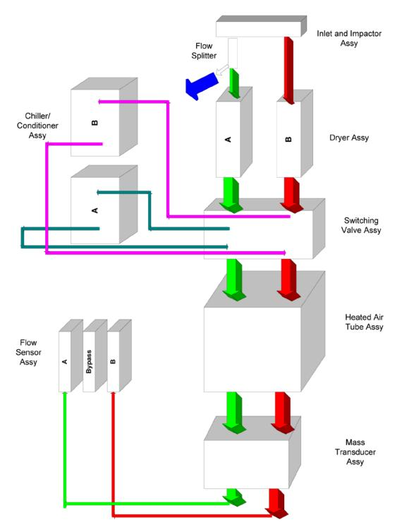
Figure 9-5. Flow paths of the fine (A) and coarse (B) streams.
