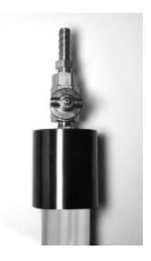
Figure 9-4. Leak check/flow adapter.
