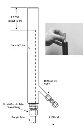
Figure 9-1. Schematic of the isokinetic flow splitter showing the position of the sample tube inside the splitter (left), which is positioned using a straight edge measure (right).
