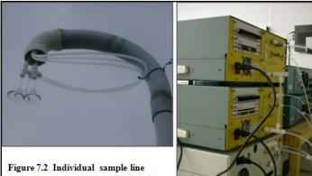
Figure 7.2 Individual sample line design for air monitoring. Probe inlet (above) and lines to back of analyzers (right)
