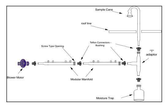
Figure 1. Conventional T-Type Glass Manifold System
