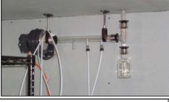
Figure 7.3 Left & top left glass intakes for manifolds; top right long tube manifold; bottom right short tube manifold with water trap.
