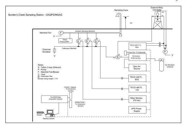
Figure 6. Example of a Manifold/Instrument Interface
