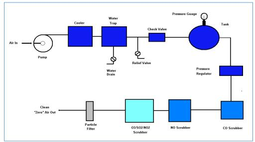
Figure 1. Diagram of a Typical Zero Air Generator System
