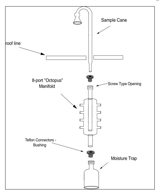
Figure 2. CARB or "Octopus" Style Manifold
