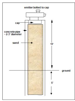
Figure 7.6 Optical mounting platform
