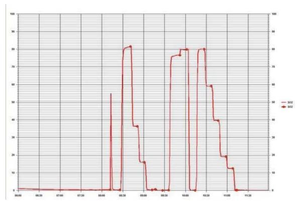
Figure 12.1 Electronic Chart Display of an SO<sub>2</sub> Calibration Procedure
