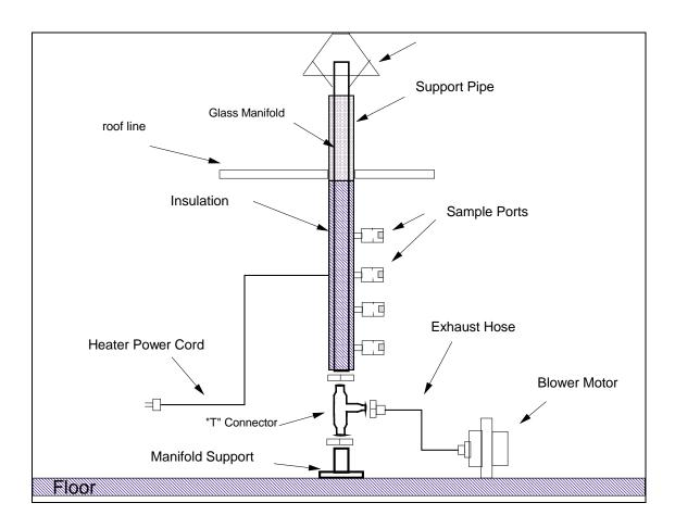
Figure 5. Example of Vertical Design Manifold
