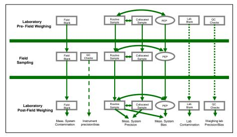
Figure 10.1 QC samples for PM<sub>2.5</sub> placed at various stages of measurement process
