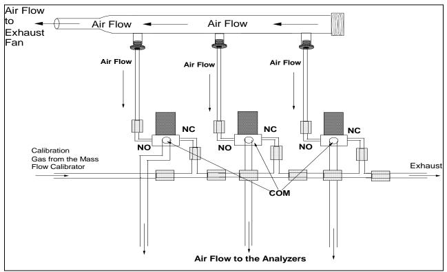
Figure 7. Ambient – Calibration Manifold Interface
