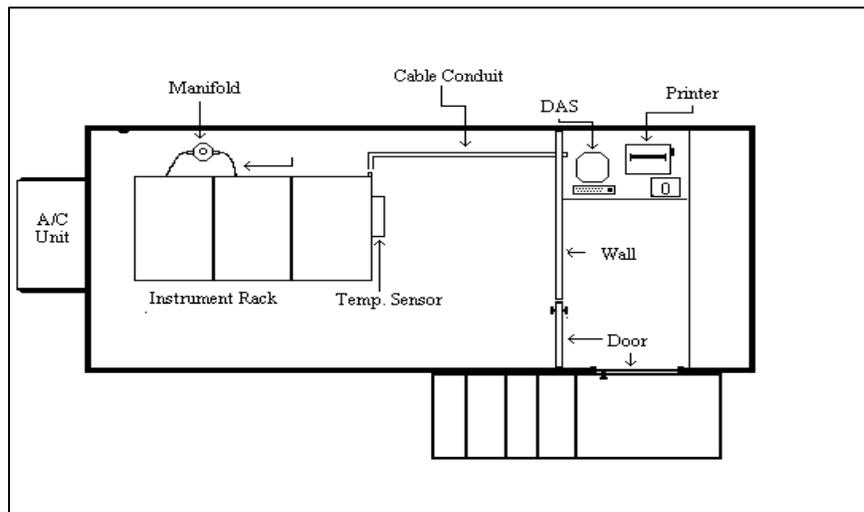
**Figure 5.1 Example design for a monitor shelter.**
