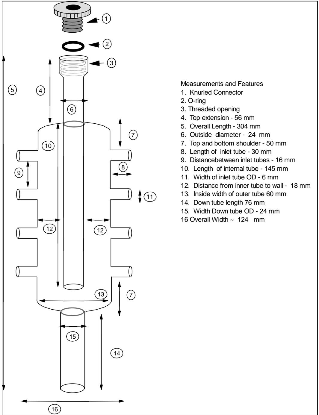
**Figure 4. Specifications for an 'Octopus' Style Manifold**
