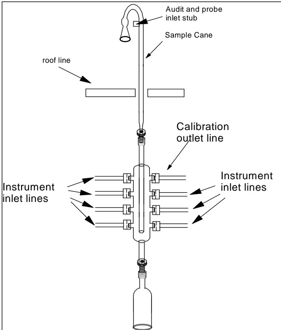
Figure 3. Placement of Lines on the Manifold
